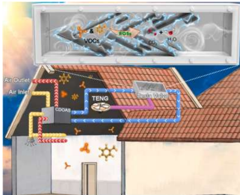
Figure 4. Schematic diagrams of the electrostatic–photocatalytic air purification system. This system is inspired by the Tesla valve, which integrates both electrostatic fields and photocatalytic purification functions [19] .
