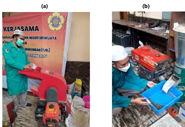
Figures 2. (a) The process of feeding rice husk into the pelletizer funnel; (b) bio-pellets product of rice husk
