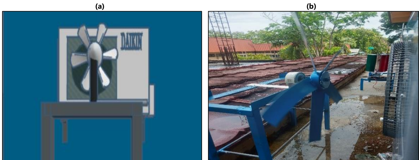
Fig 1. Turbine test scheme, (a) as a 3D drawing ; (b) actual HAWT turbine
