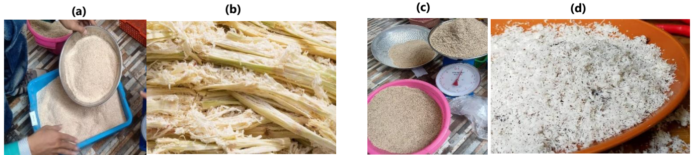
Fig 1. (a) Sugarcane bagasse after drying and chopping ; (b) Sugarcane bagasse before drying and chopping ; (c) Coconut dregs after drying ; (d) Coconut dregs before drying.
