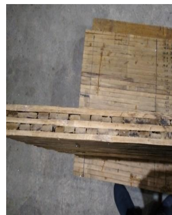
b) Breakage of CLB bamboo blades
