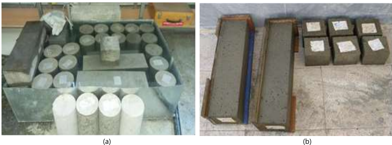
Fig.3. a) Curing and storage of concrete specimens in water tanks at 22^\circ\text{C} , b) Fresh lightweight concrete cubes and prisms with Leca-perlite mix,
