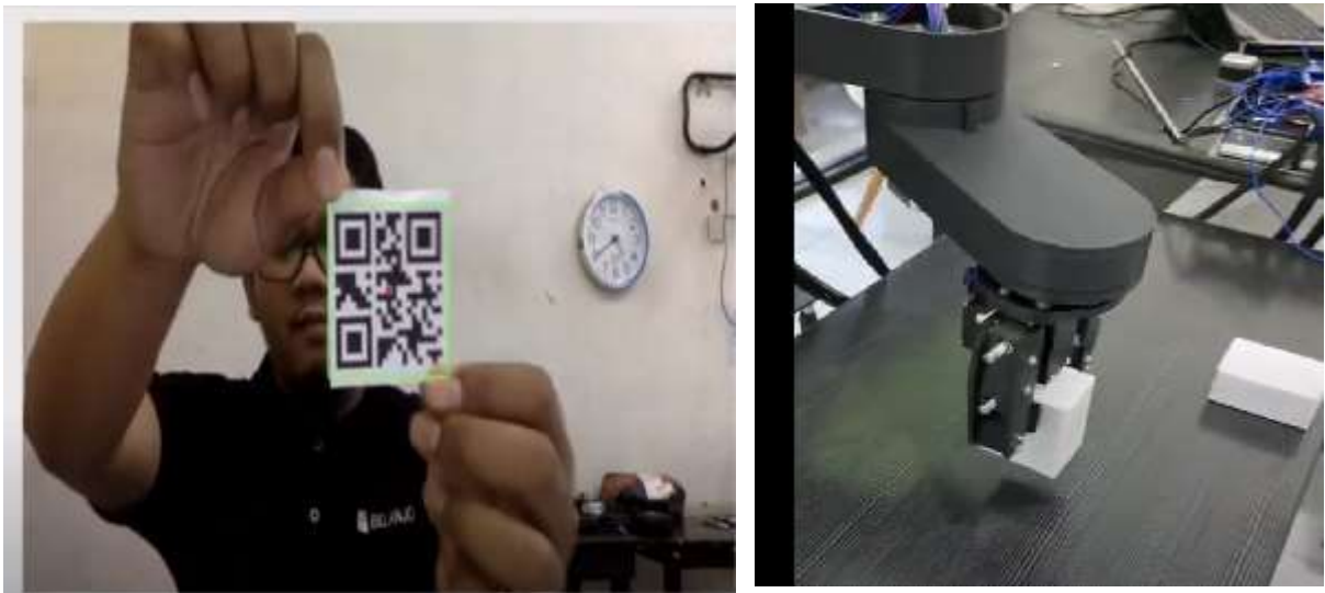
Figure 11. AI camera detection QR code
