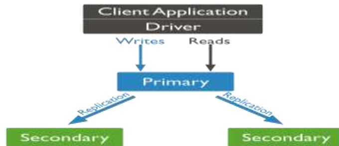
Figure 6: How does replication work in MongoDB?
