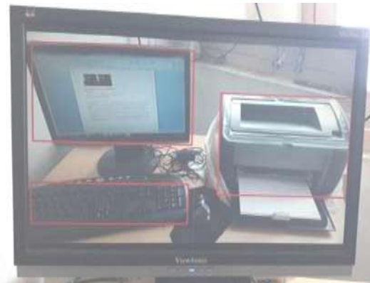
Fig 38. Output of Object detector
