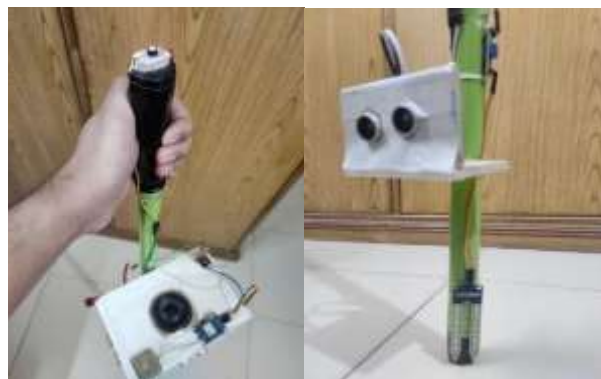
Fig 12. Fixing the Push Button and Water Moisture Sensor
