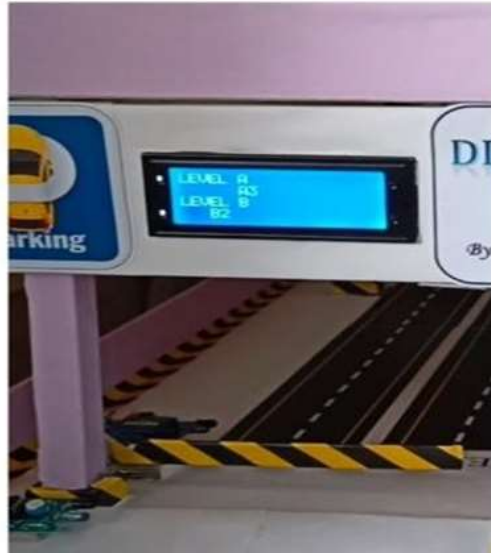
Fig. 4(b). Empty slots detected on LCD display
