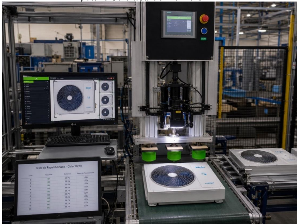
Figure 3. Image acquisition system for automated visual inspection, showing the industrial camera, lighting, fixture, logo placement, and capture environment.
