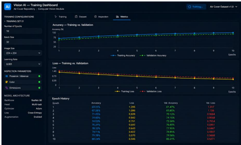
Figure 17 - Performance metrics for the computer vision model during training, showing the improvement in accuracy and the reduction in the loss function.
