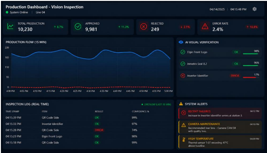
Figure 16 - Monitoring dashboard for the computer vision inspection system, showing production metrics, classification results (OK/NOK), and operational alerts.
