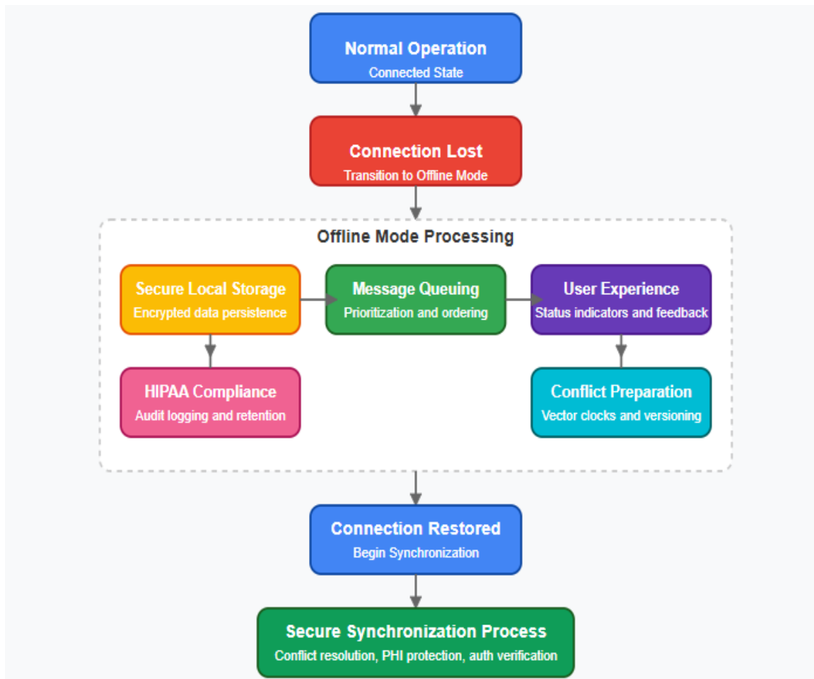
Fig. 3: Offline-First Architecture and Synchronization Workflow. [7, 8]
