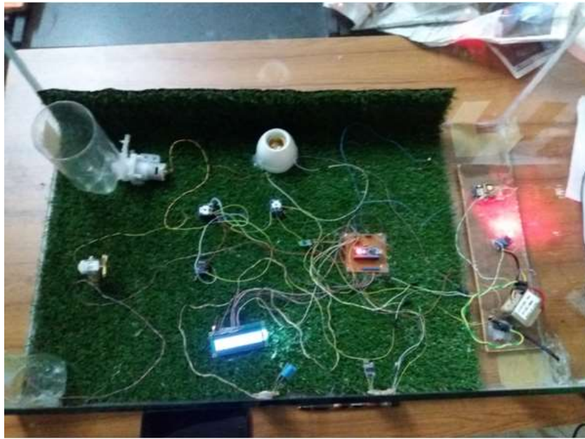
Fig. 3. Implemented prototype of the smart greenhouse.
