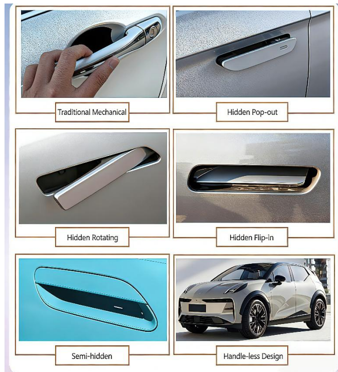
Figure 3 Hidden door handle design of new energy vehicles (from the Internet)
