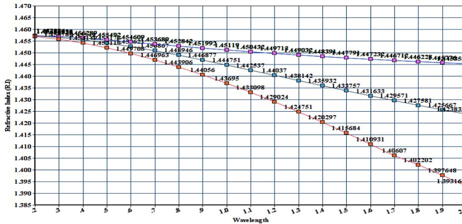
Figure: 5 Refractive Index of proposed Dual Core PCF
