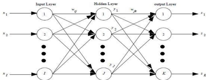
**Figure 3.** Neural network structure back propagation (baolong zhu. 2011)
